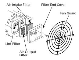
Figure 8 - Air Output, Air Intake, and Lint Filters
